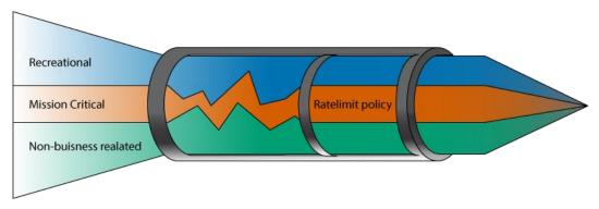
Shaping algorithms rely on timers and have the capability of delaying packets.
