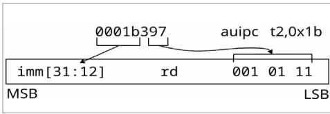
Figure 2. How auipc appears in documentation and objdump output
