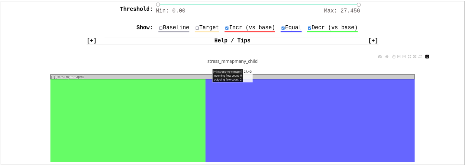
Figure 4. An interactive Sankey graph that aggregates traces into a single visualization, which allows the engineers to traverse and explore individual function traces and see how the performance changed in each function within the call chain.
